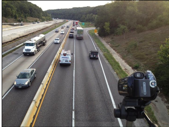
Figure 7. Video camera captures traffic directly above an overpass bridge for better processing accuracy.
